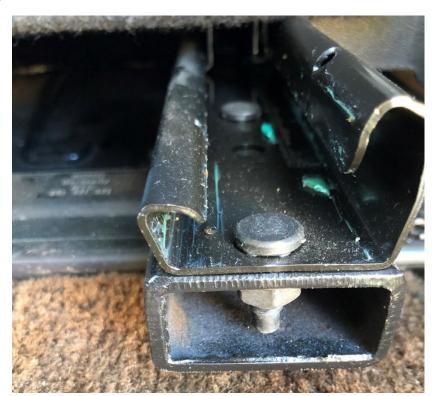
Step 3: Now you can measure the two remaining bolt locations and drill the clearance holes for these. On these two holes, drill completely through the 2"x1" and then use a step drill to open up the opposite side large enough for the socket that you will use to tighten the nut. Now you should have 3 bolt holes and 2 large clearance holes for a socket to secure the bracket to the seat.
