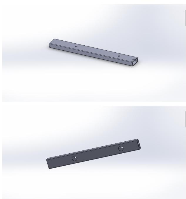
Step 4: Bolt the 2"x1" to the seat. Next step is to have you seat swivels removed and line the front of the 2"x1" with the front of the seat swivel. Make sure you are centered and straight. I then used vice grips to hold the seat swivel to the 2"x1". This allows you to drill through the swivel and the 2"x1" at the same time so you know the holes will line up. Drill these four 5/16" clearance holes on the flat part of the seat swivel.
