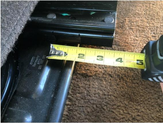
Step 7: Unbolt the adaptors completely and cut the opening. Now is the time to debur any sharp edges.
